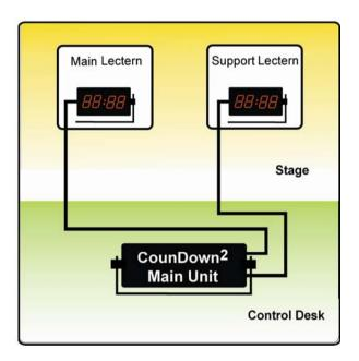
Figure 1 Connections Diagram
