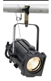
The Acclaim Fresnel is a 500W/650W general purpose luminaire (110mm diameter lens) for theatre, small studio and display lighting applications which produces an adjustable cone of light with a soft edge which is easily blended with adjacent beams to provide even illumination.
