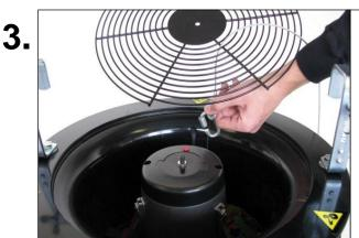
Connect a certified safety cable to the safety ring on the motor and connect the other side of the safety cable around the truss so the motor of the machine is secured to the truss.
