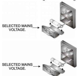
Battery charger ALTAIR WBPC-200 set up to 115 V.
